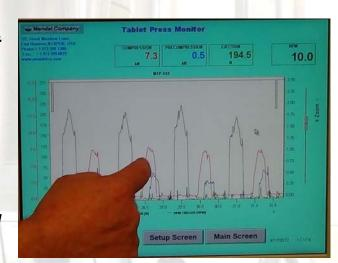
Scaled forces for Pre-Comp, Main and Ejection,
